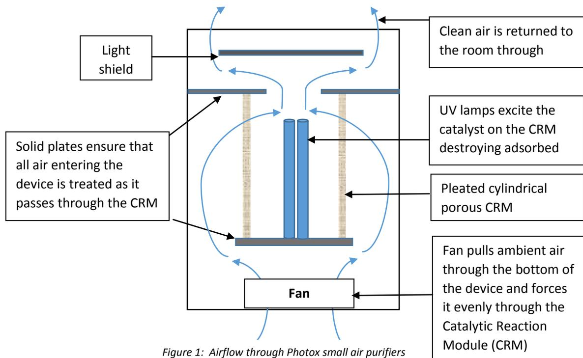
Figure 1: Airflow through Photox small air purifiers
